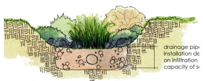
TRAPEZOIDĀL BIOSWALE other types include rectangular, triangular, and parabolic
