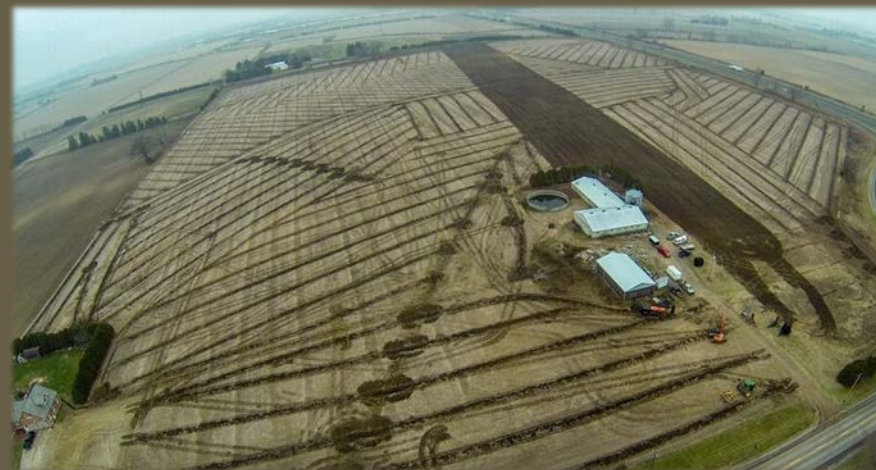
Extensive tile drainage
