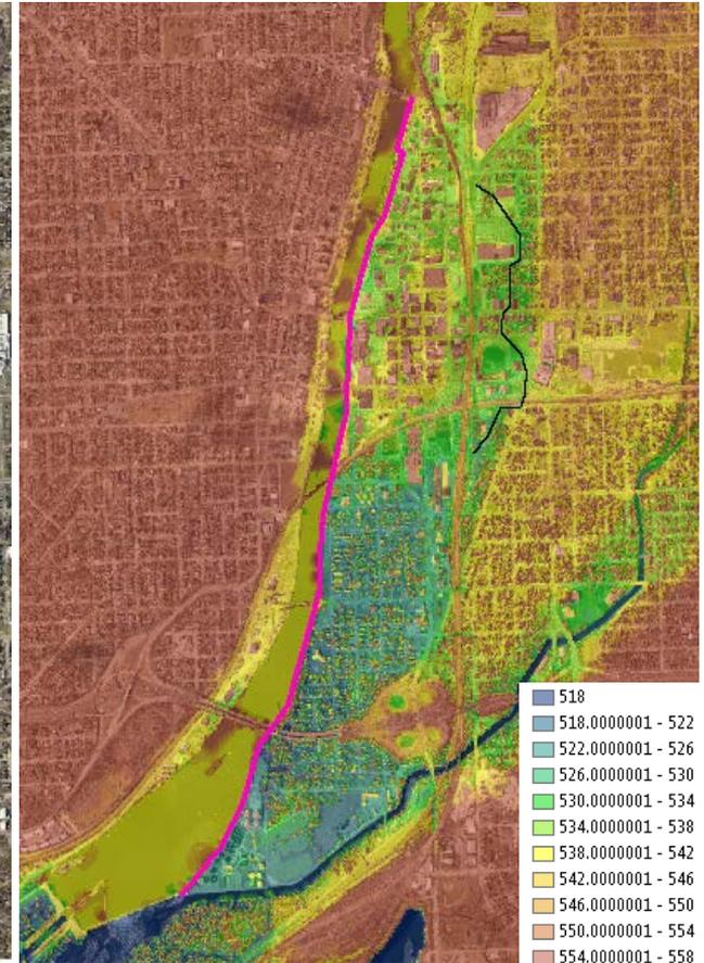
2014 LiDAR-derived DSM
