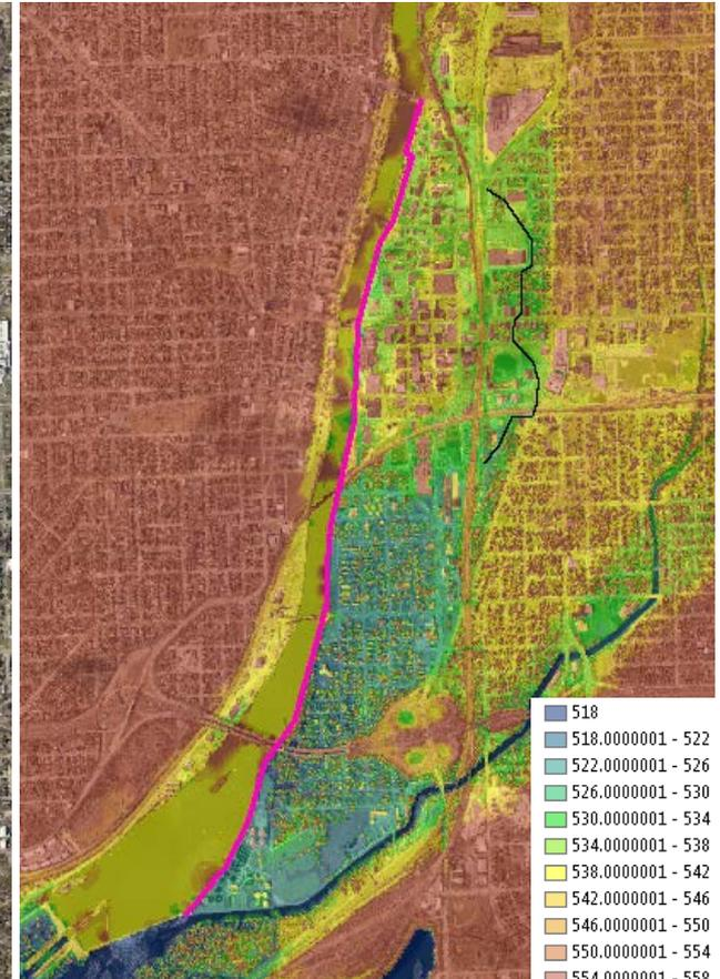
2014 LiDAR-derived DSM
