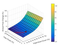
Figure 2: i-Tree Hydro simulated effects of incremental changes to Tree Cover and Impervious Cover in 161km<sup>2</sup> Rock Creek watershed near Washington, DC.
