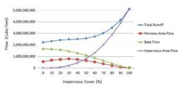
Figure 3: i-Tree Hydro simulation scaling Impervious Cover, with constant Tree Cover, in Rock Creek watershed near Washington, DC.
